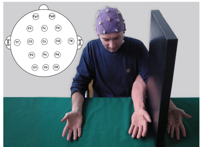
Fig. 1 The experimental set up and the 16-electrodes Biosemi cap layout. The naming scheme is taken from 10–20 international electrode placement system: Fp stands for frontal pole, F for frontal electrodes, C for central, P-parietal, and O-occipital. CMS and DLR are for the ground reference.
